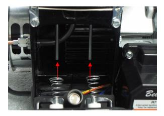
The ignitor transformer springs must contact the electrode rods when the transformer is in place and secured for operation.
