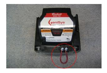
The "Tw" and "TR" terminals, normally the location of the thermostat wires, have a jumper installed to simulate a call for heat (Genisys 7505).
