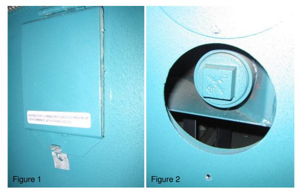
CAUTION: Be careful not to disturb the refractor material. The material becomes brittle in time and may crumble or crack if bumped by tools during cleaning or servicing.
