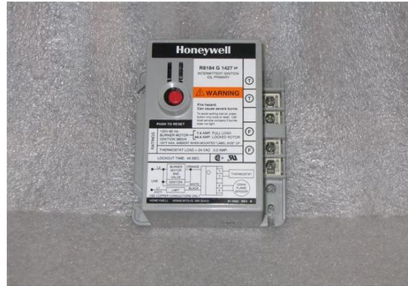
The R8184G is installed on some models. The R8184 does not have the circuitry for the pump solenoid “valve on” delay, ignition delay and purge cycle.
