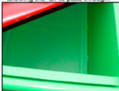
Looking down into the cart shows the specially designed screen panel that supports the soil while allowing the air to pass through.
