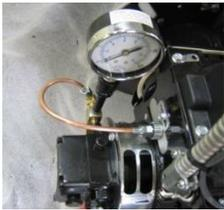
The fuel pump is factory set to 100 PSI. This insures proper atomization of the fuel. The installed gauge shows the test port location (gauge not included).
