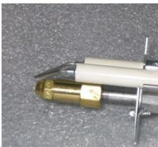
Electrodes are to be 1/16” ahead of the nozzle face, and 5/16” above the centerline of the nozzle orifice. See Beckett AFG manual for proper “F” head adjustments.
