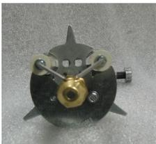
The electrodes are to be 5/32” apart. A static plate air restrictor is shown.
