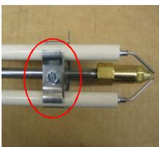
The nozzle and nozzle adapter should be tight, but not over tightened. Loosen the bolt on the electrode clamp to avoid cracking the ceramic insulators when removing the fuel nozzle
